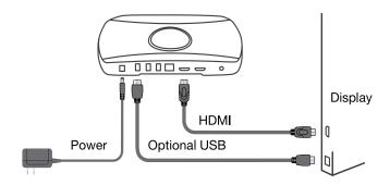
Setup is easy. All you need is your ScreenBeam wireless display receiver, power cable, HDMI cable and your display and laptop or tablet. Let's get started.
