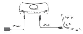
To connect with an HDMI cable, simply plug the HDMI cable into the users HDMI output port. ScreenBeam will automatically display the users screen. See the *Deployment Guide* for more information on how the hardwired connection works when a wireless session is already active. You can find the deployment guide here (click on product documentation):
