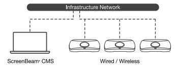
Note: Access to the LMI is prohibited by default if ScreenBeam 1100 Plus is connected to ScreenBeam CMS for management. This option can be changed in the receiver's settings.
